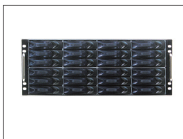
Front access 48 hard drives in 4U form factor
